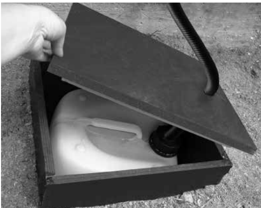
Figure 1. Seep liquid collection container
