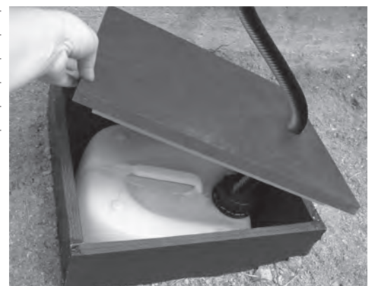
Fig. 3 Tank for collecting seep liquid
